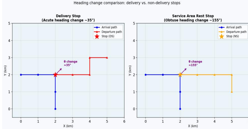
Fig. 3 Heading change at a delivery stop (left, acute turning angle approximately 35°) versus an en-route non-delivery stop such as a service-area rest stop (right, obtuse angle approximately 155°)
