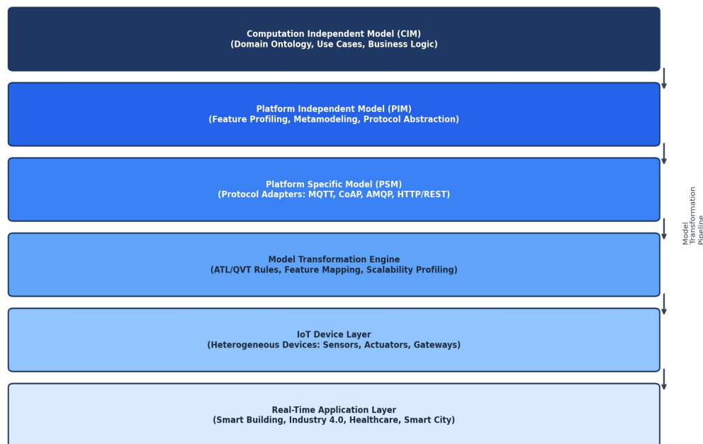
Figure 1. MDA-based IoT scalability and interoperability framework showing six functional layers from CIM domain modeling to real-time application deployment with model transformation pipeline
