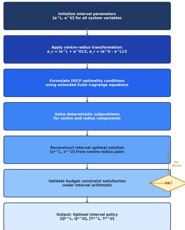
Figure 3. Improved Centre-Radius Optimization Technique (ICROT) algorithmic procedure for solving interval-valued EPQ problems
