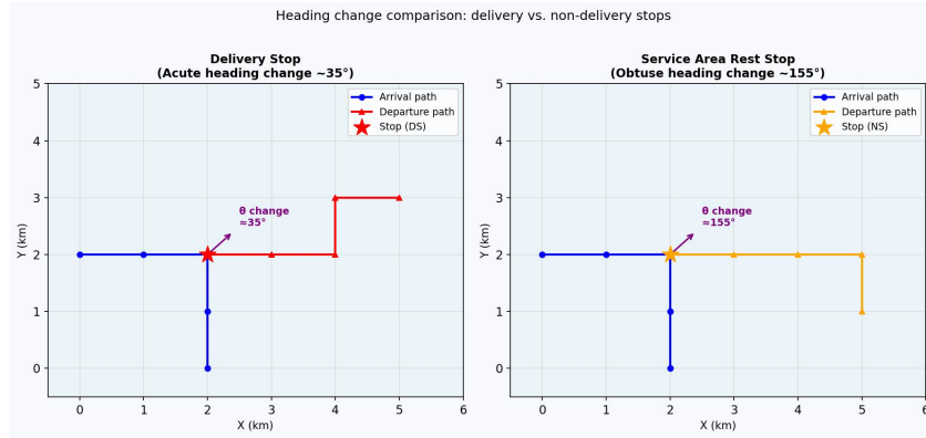
Fig. 3. Heading change patterns at delivery stops (left, acute angle \sim 35^\circ ) versus en-route non-delivery stops such as service-area rest stops (right, obtuse angle \sim 155^\circ )
