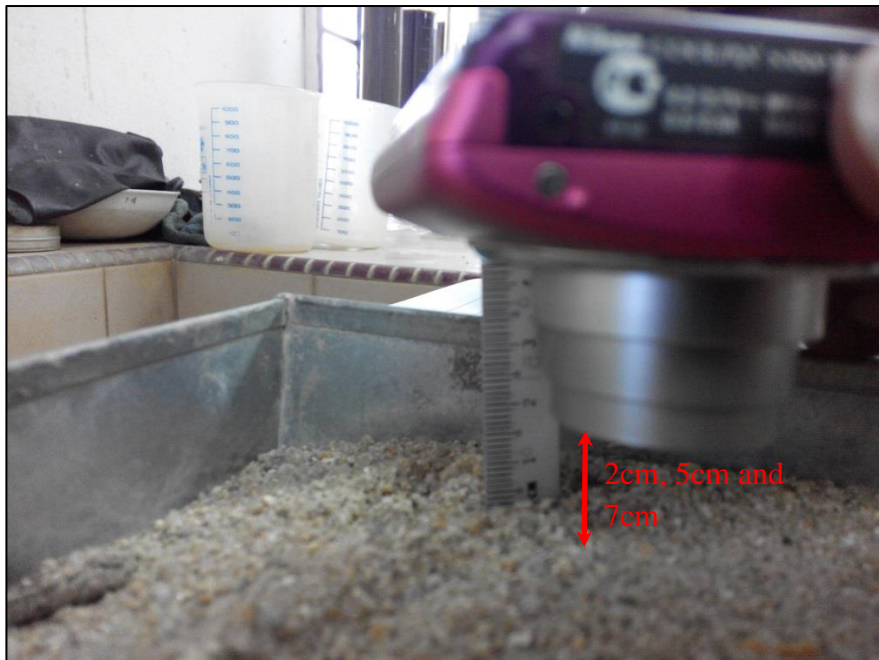
Figure 4: Distance between camera lens and sample
