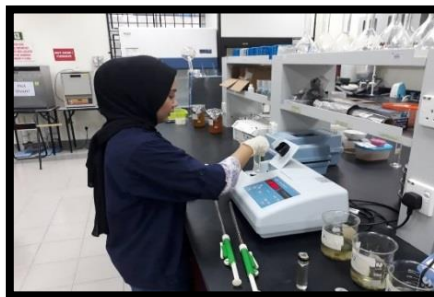
Figure 11: Turbidity results were recorded by using Turbidimeter
