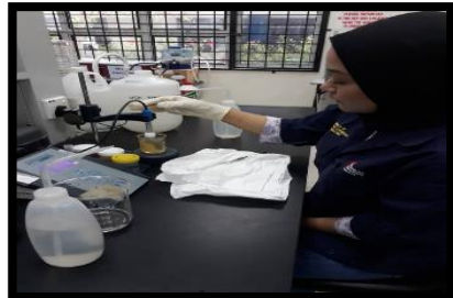
Figure 10: PH results were recorded by using pH meter
