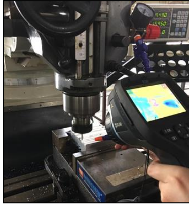
Figure 7: Capturing Cutting Temperature with Thermal Imaging Camera
