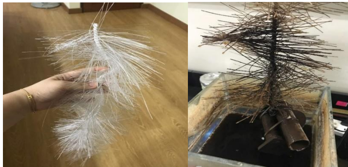
Figure 2: Colour of Attached Growth Media Changed from White Colour to Brownish Colour
