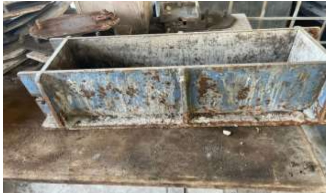
Figure 3: Beam mould 150 x 150 x 500m
