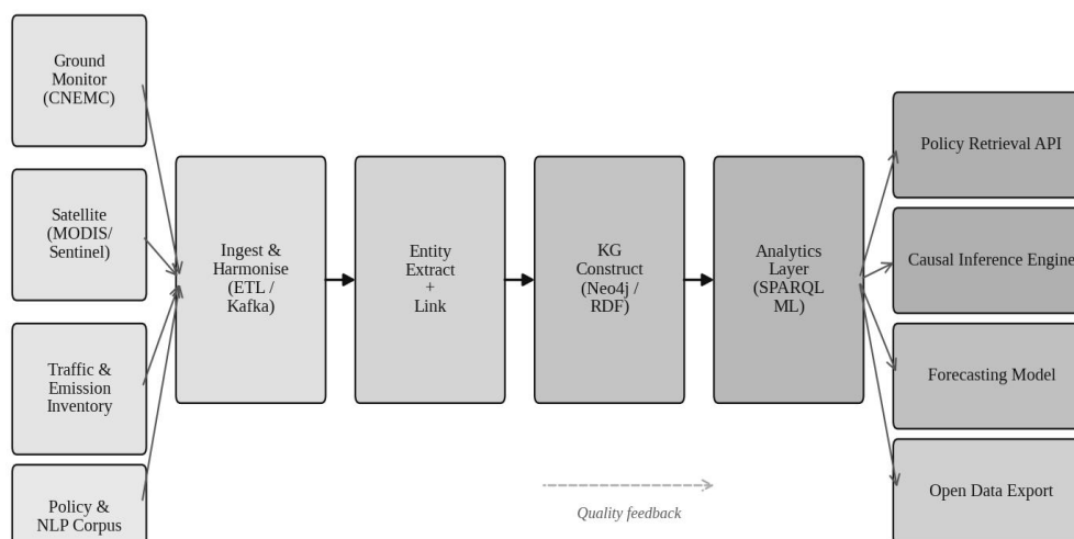
Figure 2. AirKGDB data construction pipeline. Five source streams (ground monitor, satellite, traffic/emission, weather, policy corpus) are ingested through an Extract-and-Harmonise stage, processed through Entity Extraction and Linking, loaded into the Knowledge Graph store (Neo4j / RDF triplestore), and exposed through analytics services including a SPARQL/Cypher query layer, causal inference engine, forecasting models, and open data export. The dashed arrow represents the data-quality feedback loop routing suspect records to expert review.
